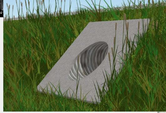
greatly improves the safety of the slope by eliminating the bulge around the headwall on the foreslope.
